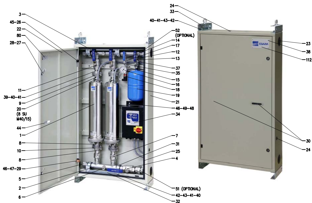
Schema componenti Cabinet Booster – Components scheme Cabinet Booster
